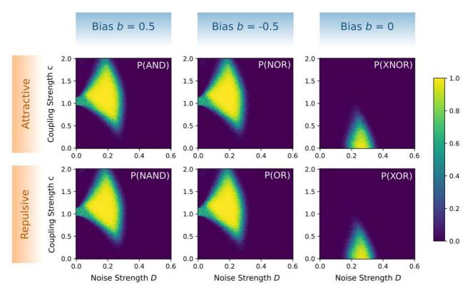
FIG. 5. Probability of obtaining reliable logic operations P(logic) for all six fundamental logic operations [P(AND), P(NOR), etc.] is plotted as a function of noise strength D and coupling strength c. The plots are made for both attractive and repulsive coupling schemes at three specific values of bias b, depicting broad regions in parameter space where all six logic operations are consistently obtained.
