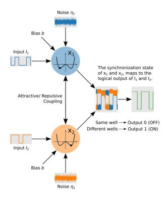
FIG. 1. Schematic representation of the concept.
